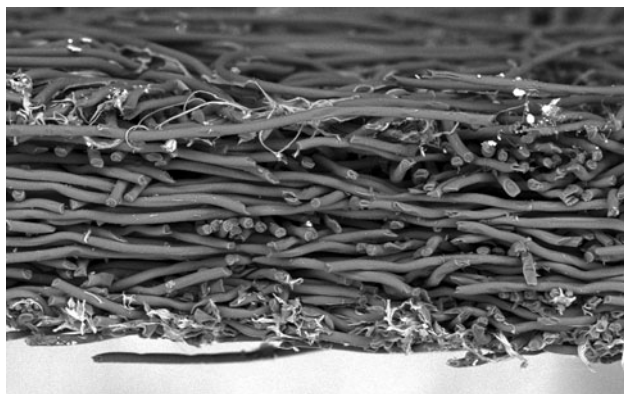
Fig. 5 Profile of a nonwoven-type GDL
